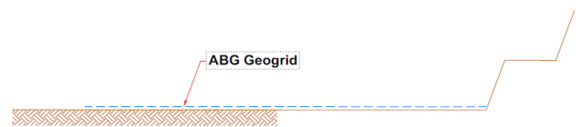
Fig. 5a: Primary geogrid is laid
