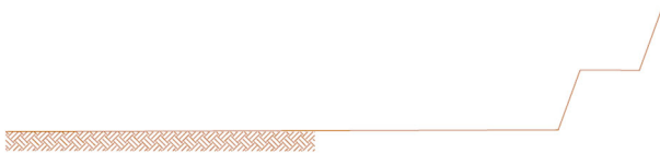
Fig. 4: Prepared formation & benching
