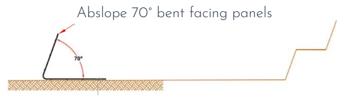
Fig. 5: Position steel panels and use 2 J pins to anchor into place at the back of the panel
