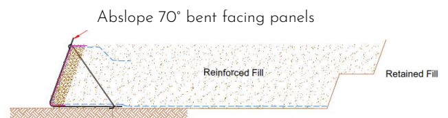
Fig. 14: Topsoil/Reinforced fill compacted and levelled to full height of facing panel
