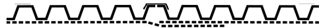
Fig. 5: Underlying geotextile flap overlap and tape joints to core on the top
