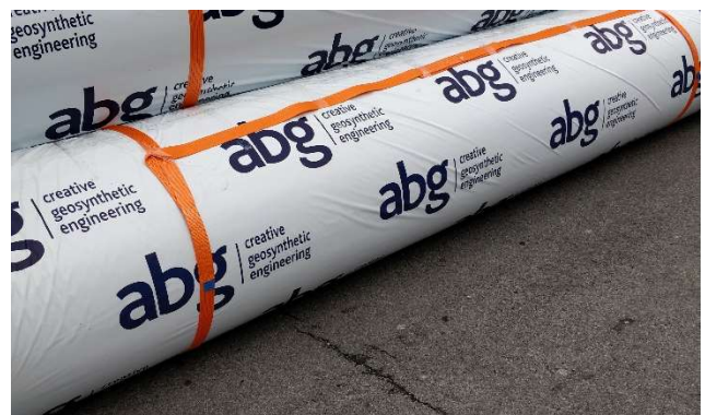
Fig. 2: Rolls supplied to site including lifting straps
