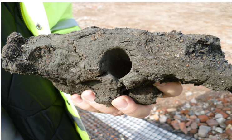
Formation: Soft river silt, high water table, CBR<1%
