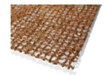
**Erosamat Type 3** is a range of permanent turf reinforcement matting products for the protection of grass roots as they establish onto steep slopes and for specification in high flow velocity conditions. The sheet is made up of a thermally bonded matrix of polypropylene fibres that create a tough, flexible and long lasting erosion control mat.
