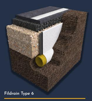
ABG Fildrain Type 6 provides vertical drainage on both sides, whilst acting as a barrier to protect the sub-base from inundation from the road verge. Fildrain Type 6 is double cuspated and fully wrapped with a filter geotextile and an integral pipe sleeve. For larger diameter pipes Fildrain 7DW[P] or 7DW[F] are applicable.
