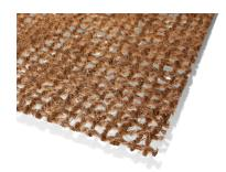
**Erosamat Type 3** is a range of permanent turf reinforcement matting products for the protection of grass roots as they establish onto steep slopes and for specification in high flow velocity conditions. The sheet is made up of a thermally bonded matrix of polypropylene fibres that create a tough, flexible and long lasting erosion control mat.
