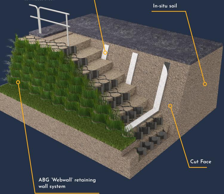
Illustrated here with ABG Webwall system but could be any reinforced earth/retaining wall solution.
