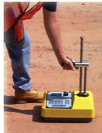
Figure 1: Nuclear density gauge
