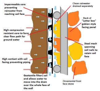
Three in one functionality: Deckdrain geocomposite provides drainage, erosion control and a barrier to rain water ingress at the front of the wall
