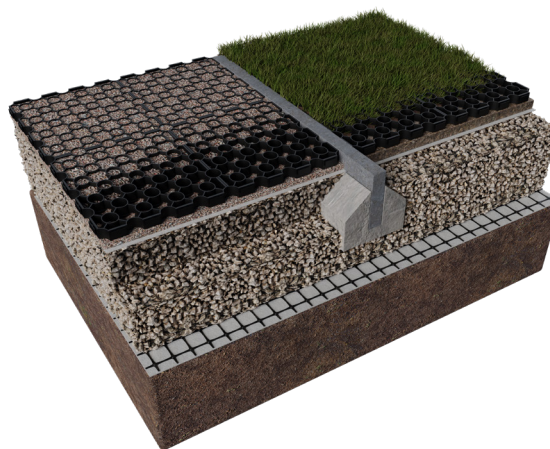
ABG Sudspave 40 permeable paver with Terrex NW9 separation geotextile
