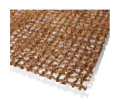
**Erosamat Type 3** is a range of permanent turf reinforcement matting for the protection of grass roots as they establish onto steep slopes and is suitable for installation above the ground cover layer. The sheet is made up of a thermally bonded matrix of polypropylene fibres that create a tough, flexible and long lasting erosion control mat.
