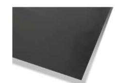
Claymat® GCL (Geosynthetic Clay Liners) are used to provide a liquid and/or gas barrier for landfill lining. Claymat provides the barrier properties of bentonite in a convenient sandwich between two layers of geotextile, needle punched together.
