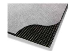
**Pozidrain®** below a capping geomembrane forms the basis of a highly-efficient gas collection and dispersal system by creating a free draining void across the cap area. Installed with the flat face of the core against the liner and dimpled face against the waste, Pozidrain also affords a high level of protection to the lining system.
