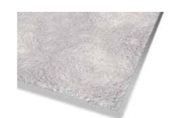
**Leakdrain®** drainage composite is designed for use as a leak detection layer between multiple linings within landfill basal containment systems. Leakdrain is available in three core thickness grades 3mm, 5mm and 6mm and in three strength grades Standard, Super and Hyper for long-term loadings up to 250kPa, 500kPa and 1,000kPa respectively.
