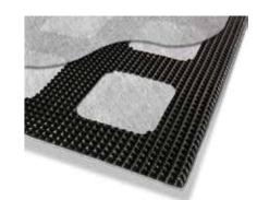
**Pozidrain® 7D** is a double-cuspated product laminated to non-woven geotextiles on both sides. It provides good long-term compressive strength whilst delivering high in-plane flow capacity in multiple directions, draining infiltration water from above and channeling away gases from below. The geotextiles allow water to freely enter the core, but prevent intrusion of the soils into the core.
