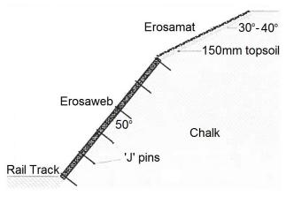
Upper slope (30°-40°) with 150mm topsoil covered by 20mm thick Erosamat. Holes drilled into the stiff chalk at the design centres across both slopes to receive the pins.
