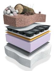
ABG Green Biodiverse Roof System with carefully selected growing media and biodiverse features overlaying the ABG Roofdrain drainage composite
