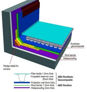
Roofdrain geocomposite combined three previously separate components into one minimising installation time
