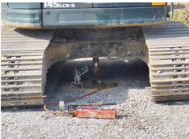
Testing after installation verified the required CBRs were achieved with the reduced material use
