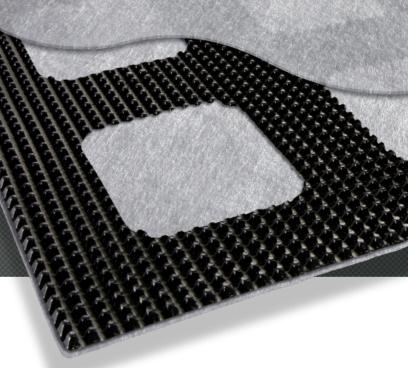
Pozidrain GSD consists of a patented lattice cuspated HDPE drainage core laminated between one or two layers of medium weight non-woven filtration/protection geotextile.
