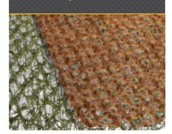
ABG offer a comprehensive range of environmentally friendly erosion control materials including biodegradable or nonbiodegradable, seeded and unseeded. They are designed to provide surface protection and enhance the structural stability of soil slopes in railway applications.
