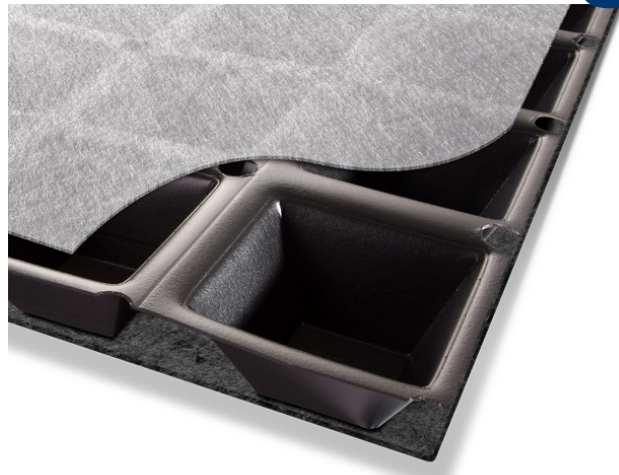
Fig. 1: Roofdrain roof drainage geocomposite, light filter geotextile on the flat side and heavier geotextile on the cusped side of the core.
