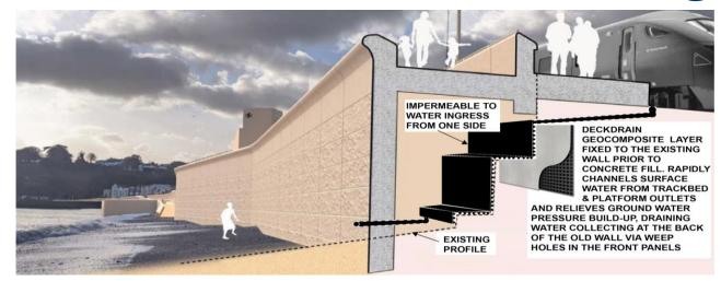
hollow concrete block drainage methods. The cuspated drainage core provides high-flow drainage capacity over a large surface area to rapidly channel surface water away from the track-bed and platform outlets. The geocomposite also prevents the fluctuating ground water pressure from building up behind the wall, with water released via weep hole outlets at the front of the new concrete panels (positioned to prevent surcharge).
