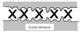
Figure 1. Soft foam applies pressure to the textile surface
