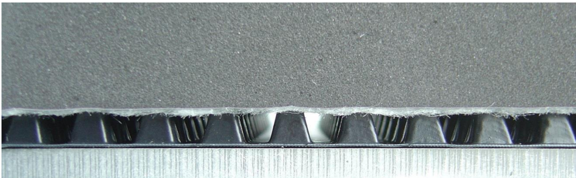
Figure 4 – Soft-Hard platen test and cuspated geocomposite at 35kPa pressure.
